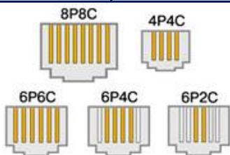
In the notation "xPyC", the letter "P" stands for 'Positions' in a plug, and "C", for "Contacts" in a socket.
