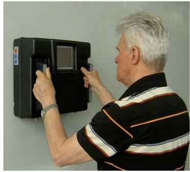
4. Turn on the radar using the button on the side of the device. The green LED lights up and the display shows controlled spaces, divided into 6 sectors and 2 half rings.
