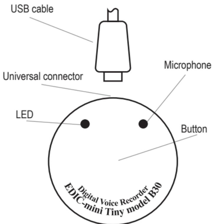
**Figure 1: Edic-mini Tiny model B30**
