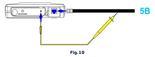
The cable is connected directly to the "INPUT" slot of the main unit. The contact with the cable shield is provided by means of the patch cord with the probe needle (Fig.1, item 22).
