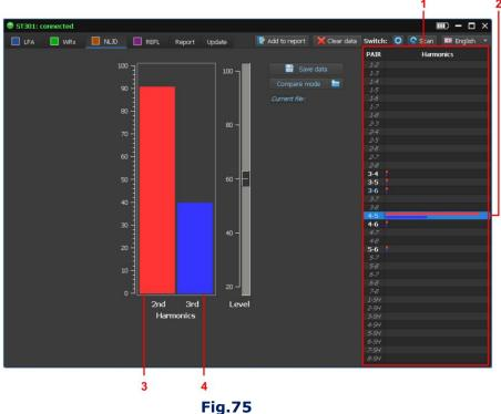
Attention! If a voltage exceeding 3 V is present in any pair of wires, the supply of the probing signal to this pair is blocked. A message appears in the corresponding row: >3V
