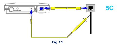
The main unit is connected to the socket by means of the patch cord (Fig.1, item 20).
