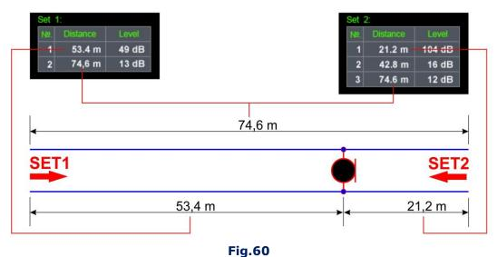
Considering the measured line length, the response obtained in the first measurement cycle at a distance of 53.4 m and in the second measurement cycle at a distance of 21.2 m are responses from the same heterogeneity.
