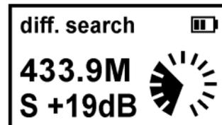
Differential Search Mode utilizes both light and sound indication of the relative signal level – the higher is the frequency of light flashing the closer is the radio transmitter.
