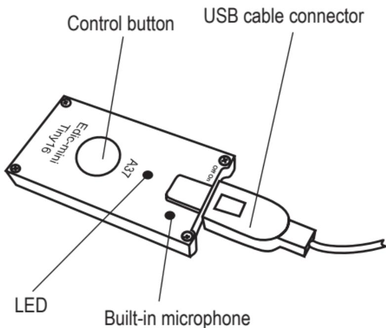
**Figure 1: Edic-mini Tiny16 Model A37**
