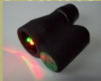
The operation principle of the device is based on the re-reflection from camera optics of light source, which emanating from the device and located on the same optical axis (light source - camera being detected - operator's eye). The angle of detection of the camera depends solely on the angle of the lens field of view of this video camera.
