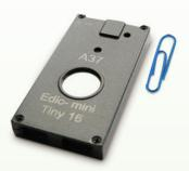
The model is designed as a tiny metal device, which won't attract much attention due to its size and design. It consumes power from a 180 mA/h Li-Pol rechargeable battery, providing continuous recording during 60 hours. The recorder has a switch of membrane type to turn the power on/off. With the help of the USB cable, which on the delivery set, you can upload the recordings from the recorder onto a computer. The recorder's case has a ring, allowing to use the recorder as a key trinket.
