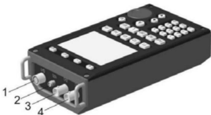
1. «I/O» Connection of UHF Converter ST131. UHF, SHF detector ST131.SHF and infrared sensor ST131.IR.
