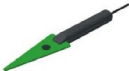
ST131.SHF consists of the log-periodic antenna and SHF detector-amplifier integrated in one body. There is a 1/4” screw hole on the handle intended to connect the tripod.
