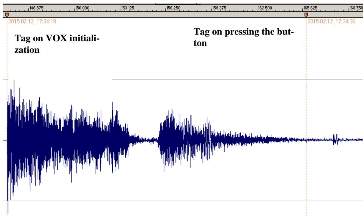
Fig. 7. Example of automatic tags recognition by the **Sound Forge** program in audio files of Soroka-16E voice recorder. The name of each label corresponds to the date and time of its creation.
