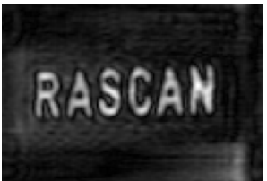
Word "RASCAN" cut from aluminum foil, under 6 cm of foamed concrete (frequency is 6.6 GHz)
