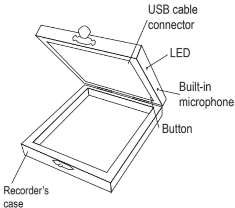
**Figure 1: Edic-mini Tiny Model A27**
