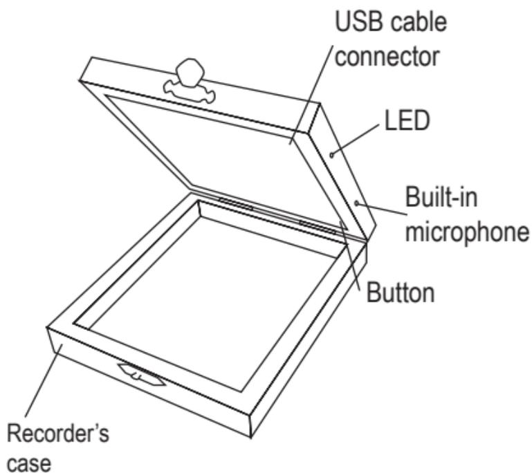
**Figure 1: Edic-mini Tiny Model A27**
