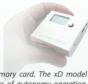
*xD model provides recording onto a replaceable xD flash memory card. The xD model is powered by a built-in rechargeable battery with up to 90 hours of autonomy operation. A high-speed card reader (USB 2.0 interface) is included into the delivery set.*
