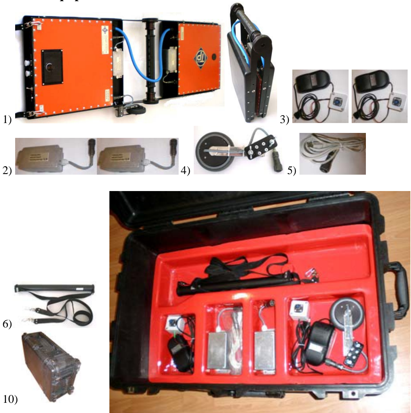
Fig.5 Set of the georadar TR-GEO-01-08 in transport case.
